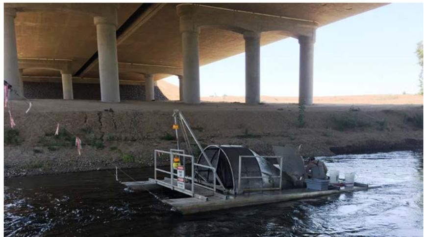
*Figure 1: Rotary Screw Trap at the Highway 99 Bridge*
