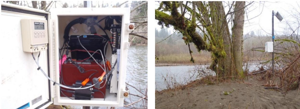
Figure 1a,b. Hydrophone installation on the Cedar River, Washington. a.) interior of the installation enclosure showing the digital timer, computer, geophone battery and charger; b.) location of the hydrophone installation (the pipe containing the cable to the hydrophone receiver is underground). Photo by M. Marineau (2/2011).
