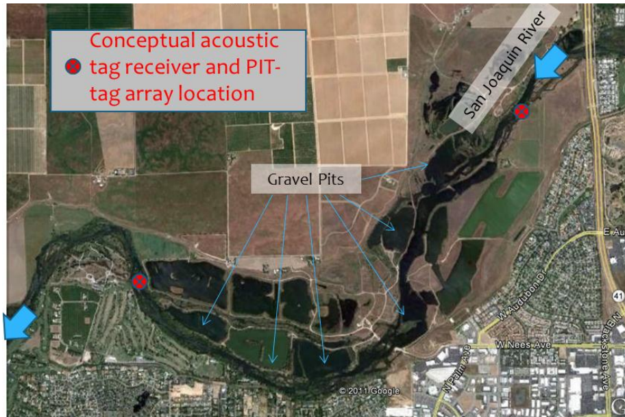
FIGURE 3: Conceptual placement of acoustic tag receivers to detect fish passage into and out of the gravel pit reach.
