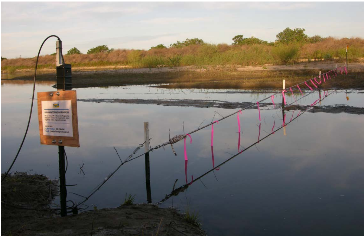
Figure 3. - Example of a swim through PIT tag antennae constructed at on the San Joaquin River, California, at the Chowchilla upstream site (Reach 2).
