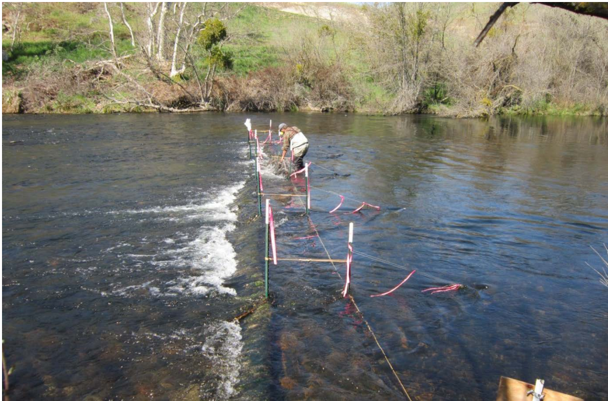
Figure 2. – Example of a pass over PIT tag antennae constructed at on the San Joaquin River, California, at the Lost River downstream site (Reach 1).
