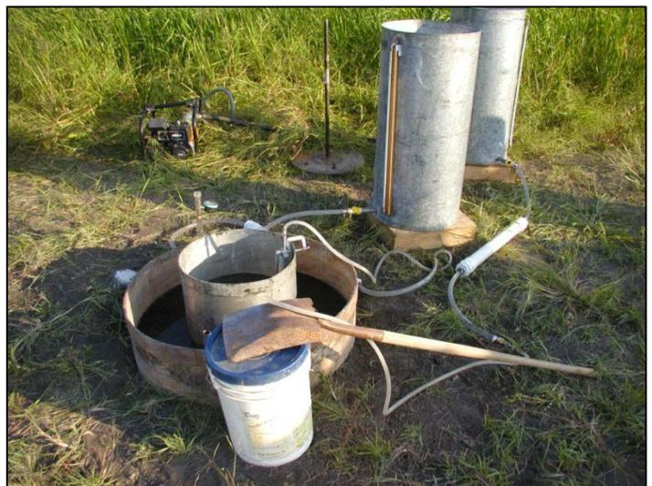
Figure 2: Shallow well pump-in test (left), and ring permeameter test (right)
