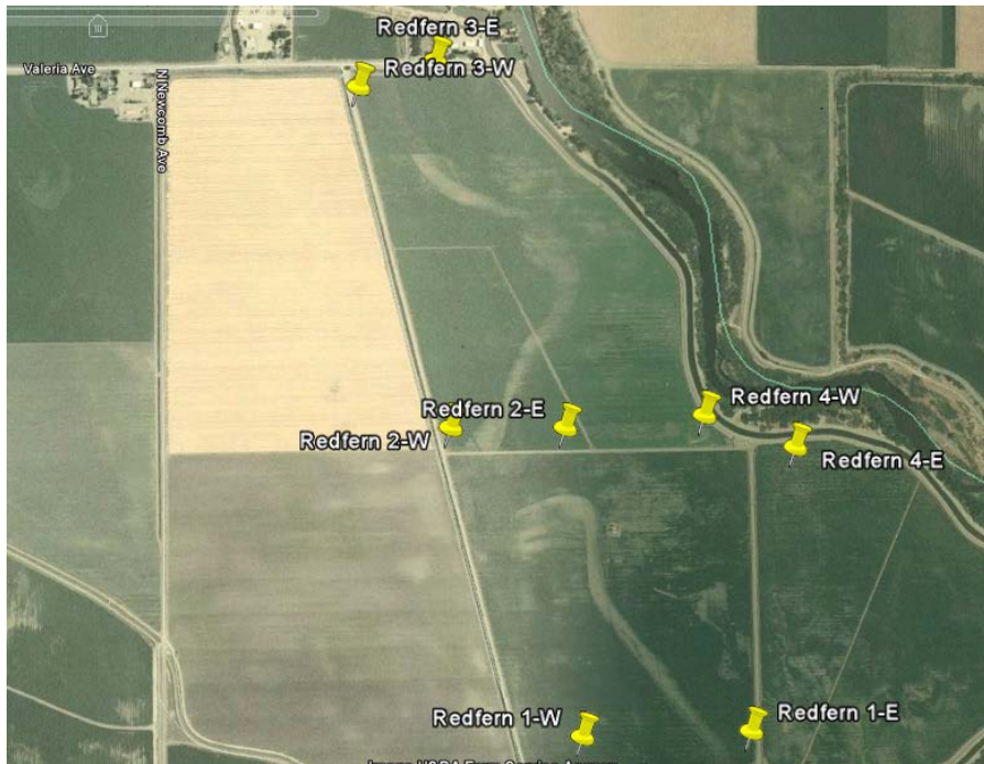
Figure 2: Property 2 Electrical Resistivity Tomography Lines
